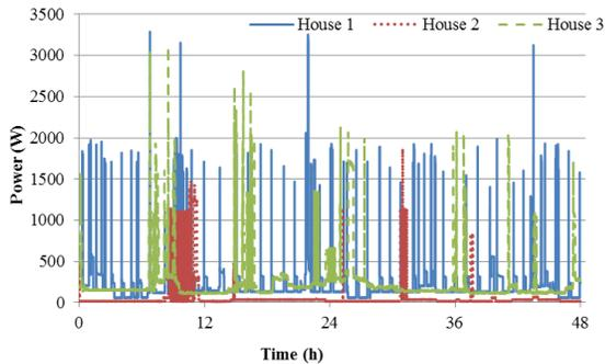
Fig. 3. Power demand profile of 3 houses from MIT REDD database [9]
