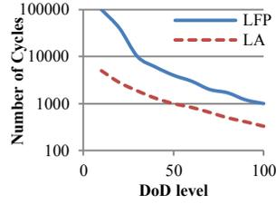
Fig.2. Cycle life of LA & LFP batteries rated at 20h [18], [19]
